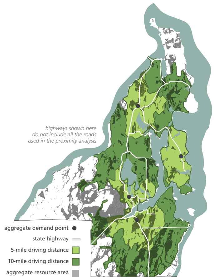
Figure 7. Proximity analysis showing a 5-mile and 10-mile outward service area from four points of aggregate demand: Port Orchard, Bremerton, Bainbridge Island, and Poulsbo.
