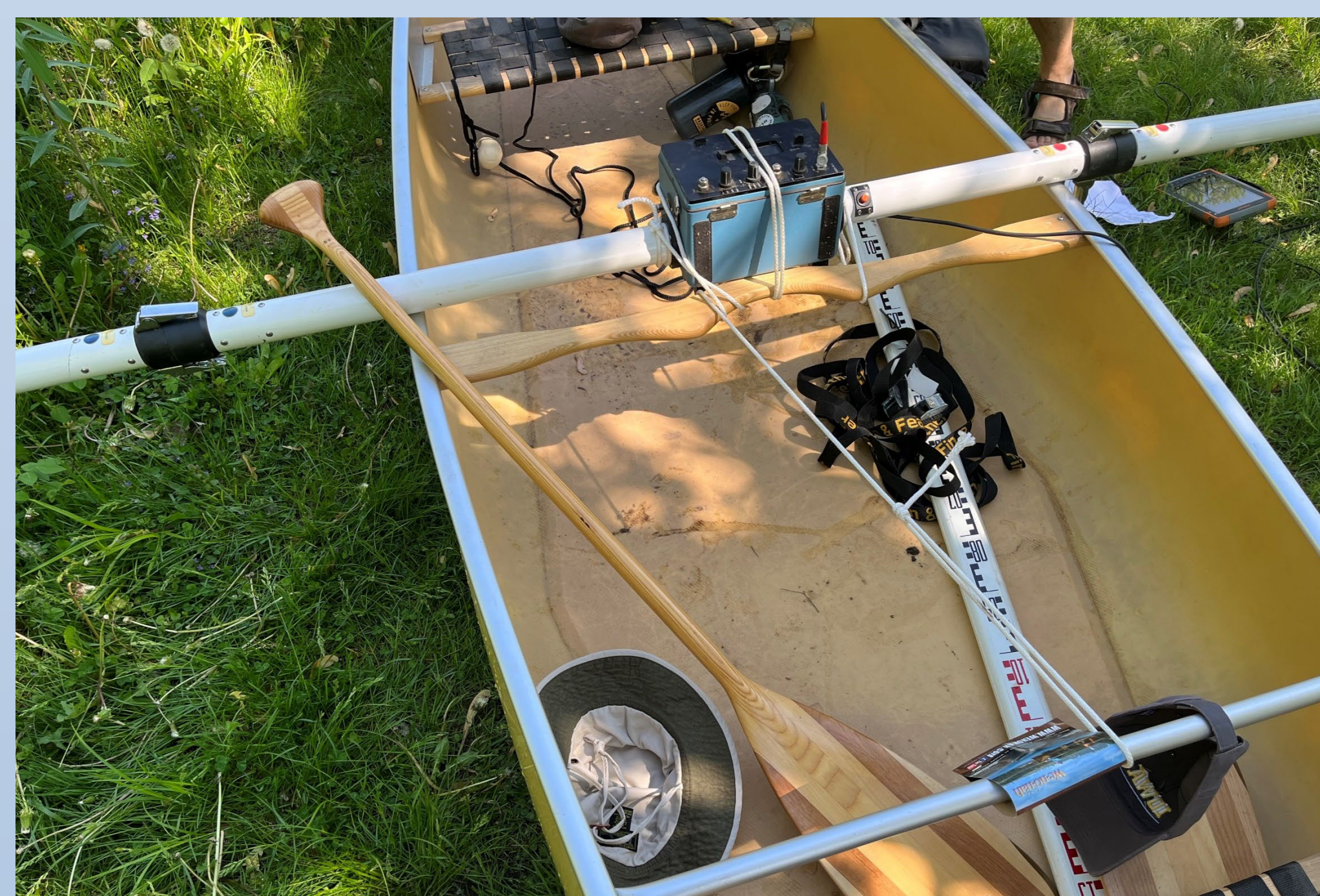
Top: A photo of the EM mounted transversely to the canoe. The photo shows the location on land where the EM was calibrated. A two-wheeled cart is shown secured to the bow of the canoe for use during portages. Bottom: A zoomed-in photo showing how the EM was secured to the canoe. Note the tablet in the grass in the upper right which was used to record continuous measurements and was connected to a sub-meter GPS (not pictured).
