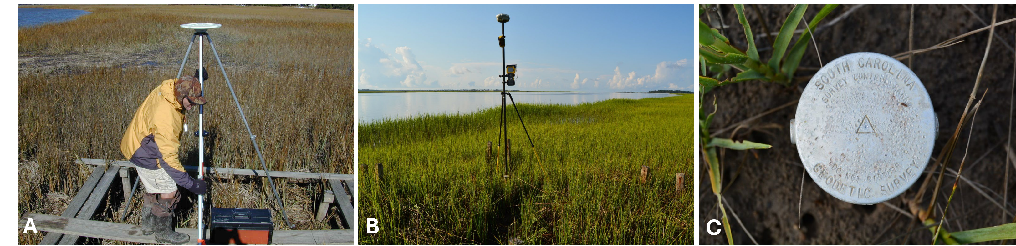
Figure 3. Geodetic data collection on SET sites evolved from base and rover (Heightmod) surveys in 1998 (A) to RTK-GNSS survey methods currently used (B). For the original SET design, a temporary benchmark cap is needed for the 3-inch aluminum pipe (C).
