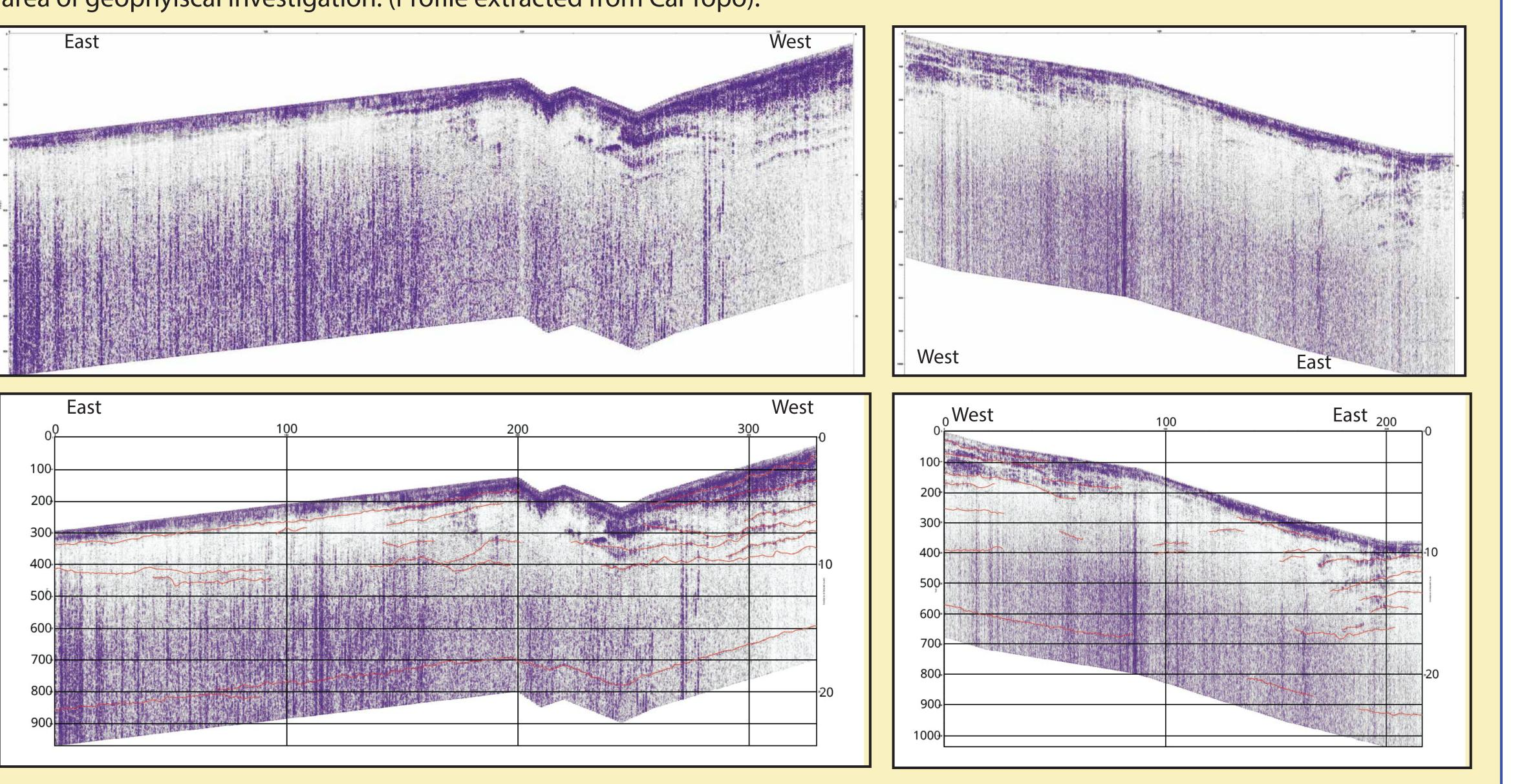
Figure 17: Radargrams for Transect 1 (left), and Transect 4 (right). Although data is still being processed and refined, the initial data show the presence of several subsurface reflectors and complex stratigraphic patterns.
