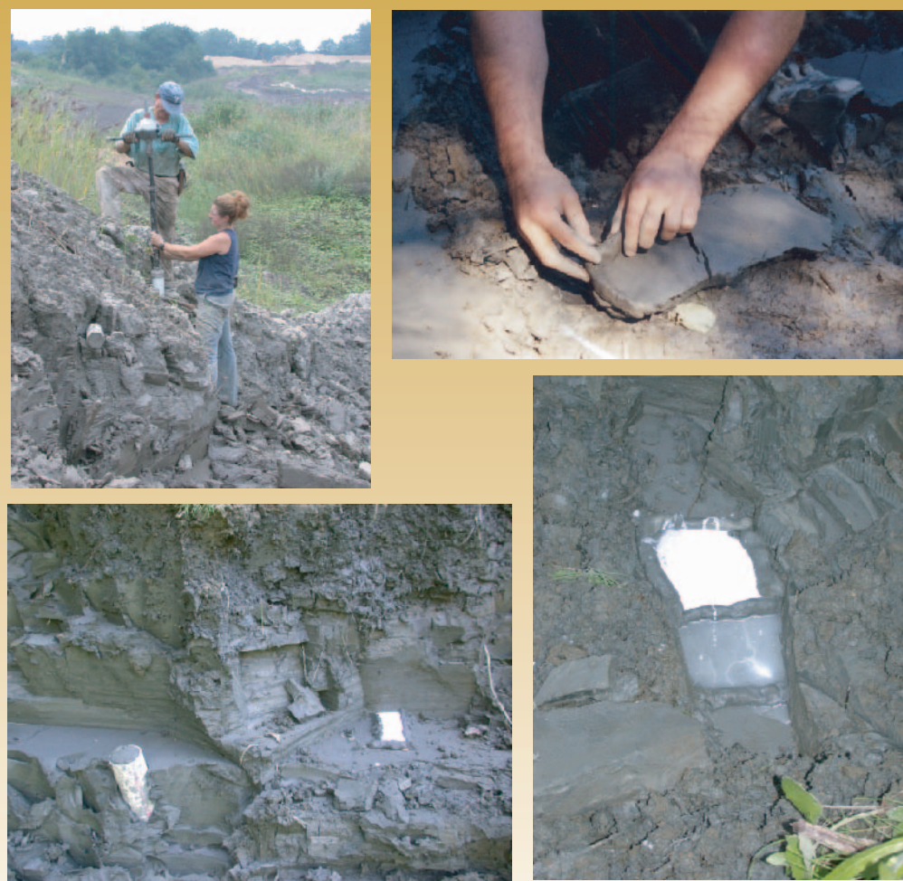
Figure 6. Clockwise from top left: 3 inch PVC cores were driven into previously unknown outcrops (K-F Brickyard, East Windsor, CT); preparation for casting an excavated block, a ring of clay was molded around the area of interest; a quick-setting plastic casting compound was poured onto the specimens; small control cores were used to locate trace fossils precisely within the section.
